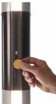
Hold the supplied magnetic wand on the marked area within the lowest black band. A red dot will illuminate on the display to show that the system is active. Keep the magnet in place for around 10 seconds when the display will illuminate to show the current lighting level. Swiping the magnet across the area will advance the lighting level making the post brighter. When level 7 is reached, a further swipe will return to setting 0.
